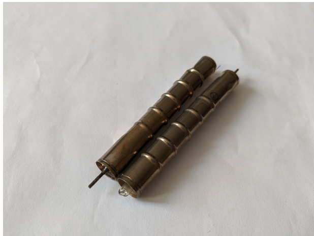
Figure 2: SBM-20 tubes with exposed leads. The protruding rod is the anode and the tube body is the cathode
